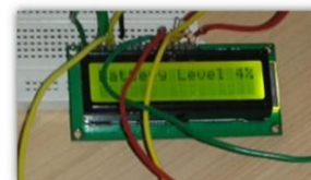
Fig. 26. Battery Level of phone displayed on LCD
