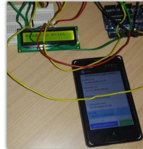
Fig. 24. Pairing Android application with HC05 Bluetooth
