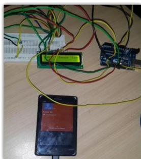
Fig. 27. Notification of call displayed on LCD
