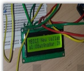
Fig. 28. Current location of phone displayed on LCD
