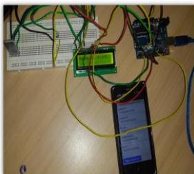
Fig. 23. Android application searching Bluetooth device will be displayed on lcd. here we see the name of the calling person.
